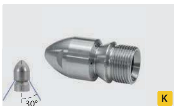
M22x1.5 M. Outside \varnothing 25 mm. rear jets
