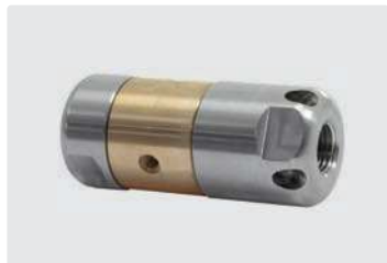
1/4" F. rear jets. 3 side jets. Outside Ø 30 mm.
