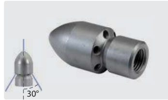
1/4" F. Outside \varnothing 25 mm. rear jets, with front jet
