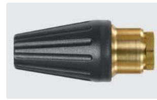
1/2" F. Spray angle 20°. 120 - 250 bar. Max. 100 °C
