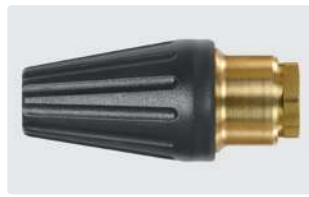
1/2" F. Spray angle 20°. 120 - 250 bar. Max. 100 °C
