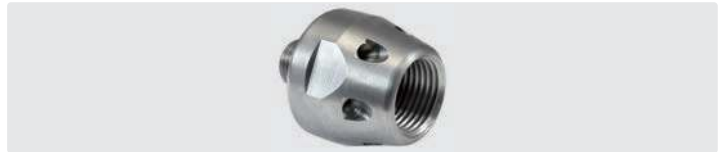
Hardened stainless steel. 6 M5 threads for nozzle inserts (see table below)
