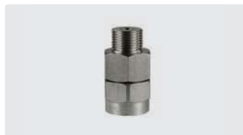
3/8" M : 3/8" F. Stainless steel. Max. 500 bar / 90 °C
