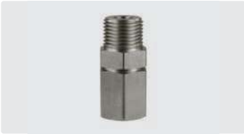
1/2" M : 1/2" F. Stainless steel. Max. 350 bar / 90 °C
