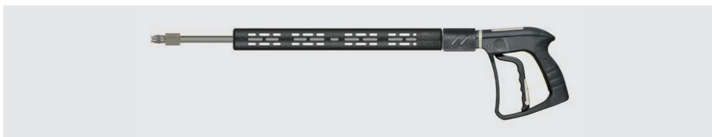
Professional steam gun ST-4000 with lance 500 mm stainless steel with vented handle ST-9 380 mm and steam low pressure nozzle made out of stainless steel. Max. 20 bar / 200 °C
