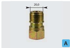
Plug : F. Zinc-plated steel. Max. 250 bar / 150 °C
