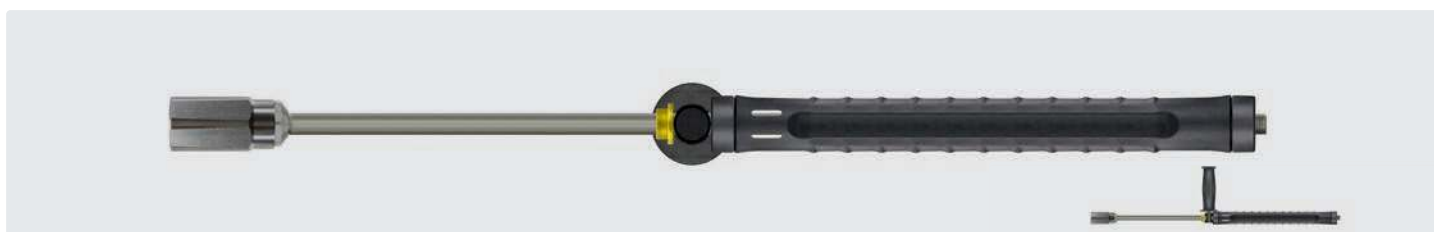
1/4" M. Foam lance stainless steel with air injector, vented handle ST-9.9 330 mm, grip and stainless steel socket with nozzle. A foam injector is required. Max. 250 bar / 80 °C
